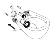
$\rm e)$  . Fasten the cone-shape screw through the installation hole on toilet cover by Allen key.
